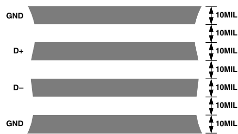
Figure 6. Arrangement of Signal Tracks
